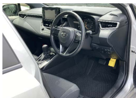
Compact wireless communication module connected to vehicle
