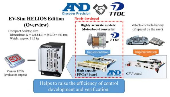
\* A FPGA (field programmable gate array) is the name of a freely programmable electronic device in a digital circuit.
