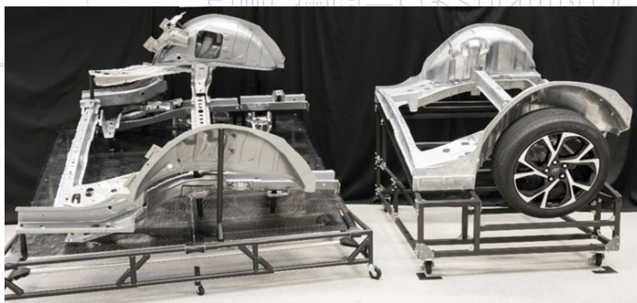
(Left) Conventional stamped structure (Right) Giga cast structure (Source: TMC)
