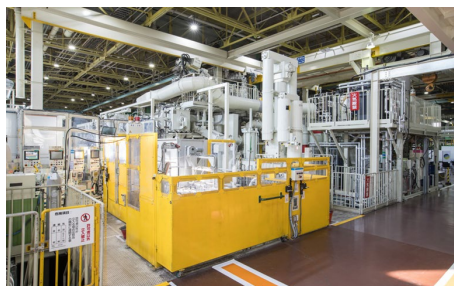
Myochi Plant: Die casting machine for prototypes (source: TMC)
