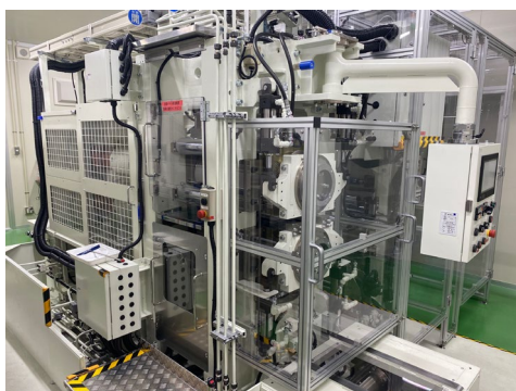
Roll press installed in a dry environment
